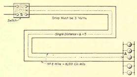
Fig. 93.—Arranging circuit to have a given drop.
